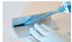
After work finish or during breaks, the mixing tube can remain on the cartridge as closure instead of the original closure cap.
