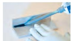
After work finish or during breaks, the mixing tube can usually remain on the cartridge as closure instead of the original end cap.
